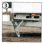
Move the support legs down so the trailer is horizontal. The angle should be at least 45 degrees from the trailer.
