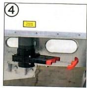
Pull the handle to empty the toilet tank. Flush through with water to clean it.
