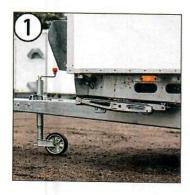
Prepare the trailer for driving (see disconnecting). Move down the nose wheel and move the support legs up.
