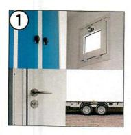
Close and lock cupboards, windows and doors. Secure any loose parts and place heavy objects over the axle.
