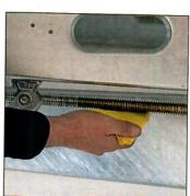
Use a spray or cloth to lubricate the 4 spindles for the support legs.
