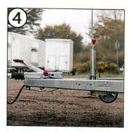
Move the nose wheel up and release the handbrake. Check that there are no cables touching the ground.
