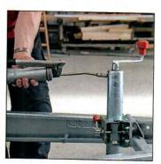
Use a grease gun to lubricate the 3 grease nipples on the overrun brake and jockey wheel.
