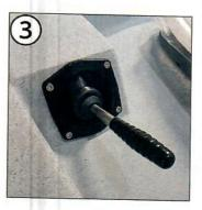
Pump the handle on the side of the toilet to flush the toilet with water.
