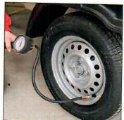
The wheel rims must be tightened with a pressure of 90 Nm (9 kilo). Pump the tires according to numbers on the tires.
