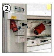
Find the electrical inlet. It will be in the technical compartment or on the side of the chassis under the trailer.
