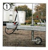
Put the handbrake on and move the jockey wheel down. Remove the electrical socket and safety wire. Then release the trailers.
