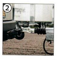
Place the ball connection on the pull ball. Press the handle down and check that it is placed correctly (click sound).
